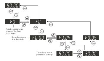
Figure 3-2 parameter queryand modification process
